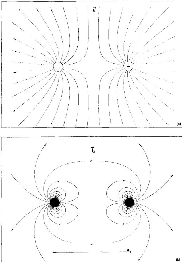
Fig. 5. (a) Sketch of the electric field lines in a plane perpendicular to the (parallel) axes of two equally and similarly charged cylinders. (b) Sketch of the  $j_x$  stream lines in the electrostatic field of Fig. 5(a). If the sense of direction of the stream lines is reversed, this becomes the sketch of the  $j_x$  stream lines in the magnetic field of two attracting line currents.
