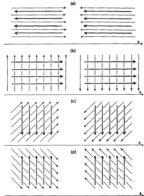
Fig. 2. Illustration of some rules useful for sketching the direction of the  $\mathbf{j}_x$  stream lines (heavy lines) for various orientations of  $\mathbf{E}$  (light lines): (a)  $\mathbf{E}$  parallel or antiparallel to the  $+x$  direction. (b)  $\mathbf{E}$  parallel or antiparallel to the  $+y$  direction. (c)  $\mathbf{E}$  makes an angle of  $+\pi/4$  or  $-3\pi/4$  with the  $+x$  direction. (d)  $\mathbf{E}$  makes an angle of  $-\pi/4$  or  $+3\pi/4$  with the  $+x$  direction.
