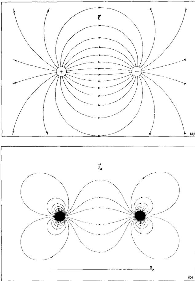
Fig. 4. (a) Sketch of the electric field lines in a plane perpendicular to the (parallel) axes of two equally but oppositely charged cylinders. (b) Sketch of the  $j_x$  stream lines in the electrostatic field of Fig. 4(a). If the sense of direction of the stream lines is reversed, this becomes the sketch of the  $j_x$  stream lines in the magnetic field of two repelling line currents.
