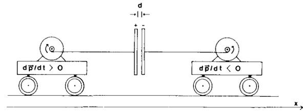
Fig. 1. Two wagons are connected across the plates of a capacitor by means of two ropes. The wagons are being pulled together with the help of motors attached to each wagon. For simplicity of argument, the motors are assumed to be winding up the ropes around spools in such a way that the separation between the capacitor plates remains constant throughout the process.
