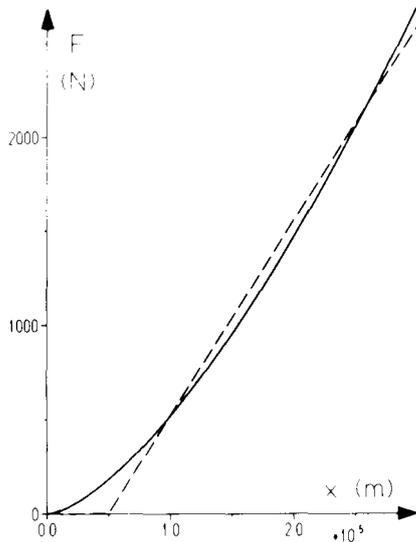
Fig. 2. Force  $F$  as a function of the deformation  $x$  in one dimension for a steel ball, 5 cm in diameter, according to the theory of Hertz (solid line). The dashed line represents an approximation of this curve by two straight lines.
