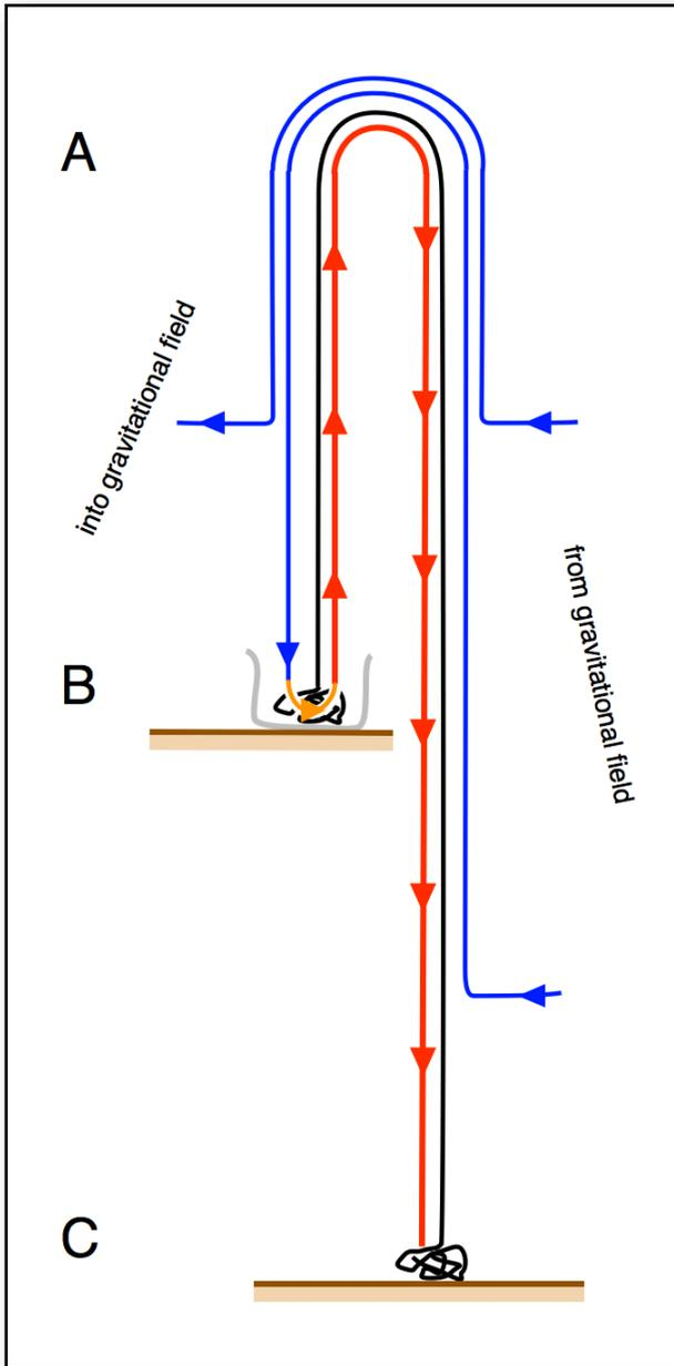
It is flowing upwards, turns left together with the chain and goes down again. It is available for the acceleration of the beads in the container at position B.
