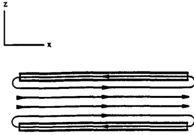
Fig. 2. Half of the energy which is moving within the field from left to right flows back to the left through the plates of the capacitor.
