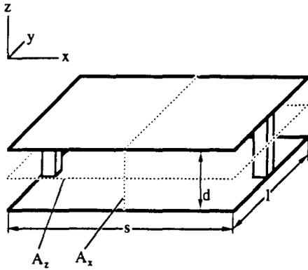
Fig. 1. When the capacitor is moving upward, energy is flowing through the spacers from the lower to the upper plate. When the capacitor is moving to the right, energy is flowing through the plates from right to left.
